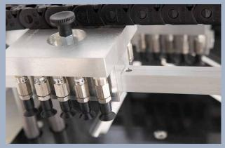
Pickup head for the optional stack loader.
