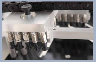
Pickup head for the optional stack loader.
