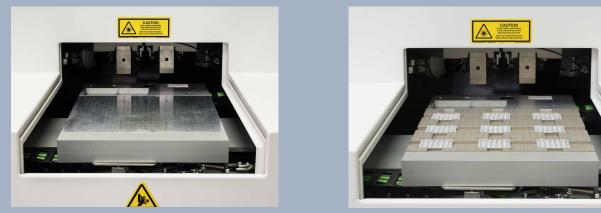
Standard flat vacuum chuck on the left and a custom fixture on the right for a 3x3 array of substrates.
