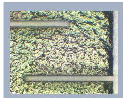
Two plunges of a serpentine trim in thick film material.
