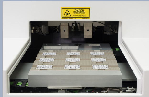
Custom fixture for a 3x3 array of substrates.
