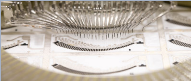
Probing arrangement for fuel gauge sensor.
