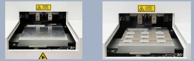
Standard flat vacuum chuck on the left and a custom fixture on the right for a 3x3 array of substrates.
