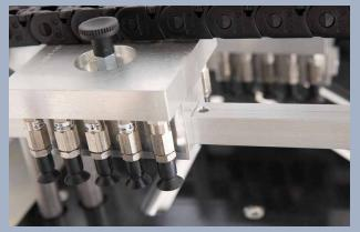
Pickup head for the optional stack loader.
