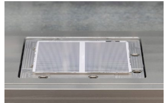
Substrate with array of RTDs on the temperature-controlled vacuum chuck.
